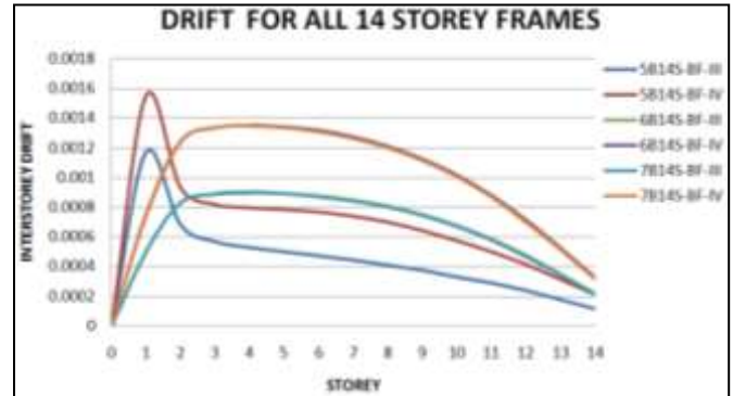
Fig. 2: Storey Drift Comparison for All Fourteen Storey Bare Frames
