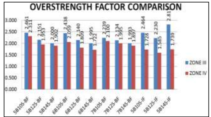
Fig. 10: Effect on Overstrength Factor Due To Change in Seismic Zone
