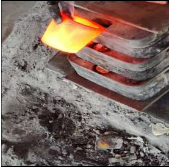
Fig. 2: To produce the final specimen, sand-casting is being done.
