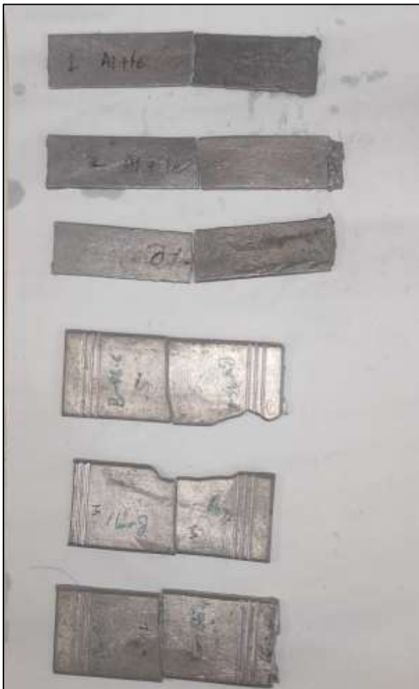
Fig. 3: show the samples of Al+Fe and Al+Fe+Bronze after testing produced by sand casting method
