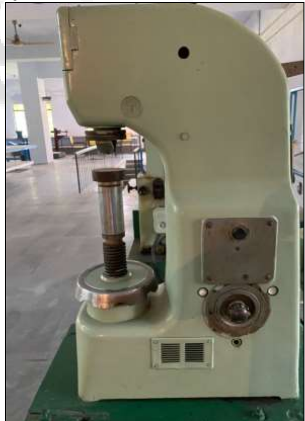
Fig. 4: Shows the Rockwell hardness testing machine
