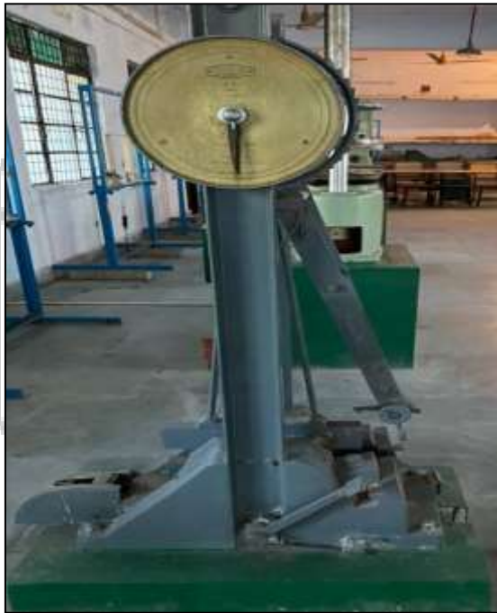
Fig. 5: Show the Charpy impact testing Machine
