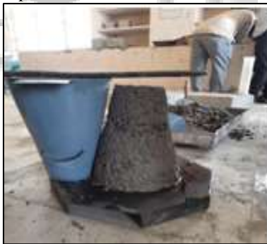
Fig. 3.1: Slump cone test
