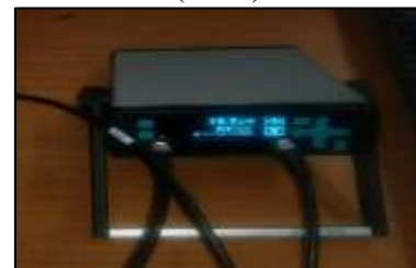
Fig. 3.3: Ultrasonic pulse velocity test setup
