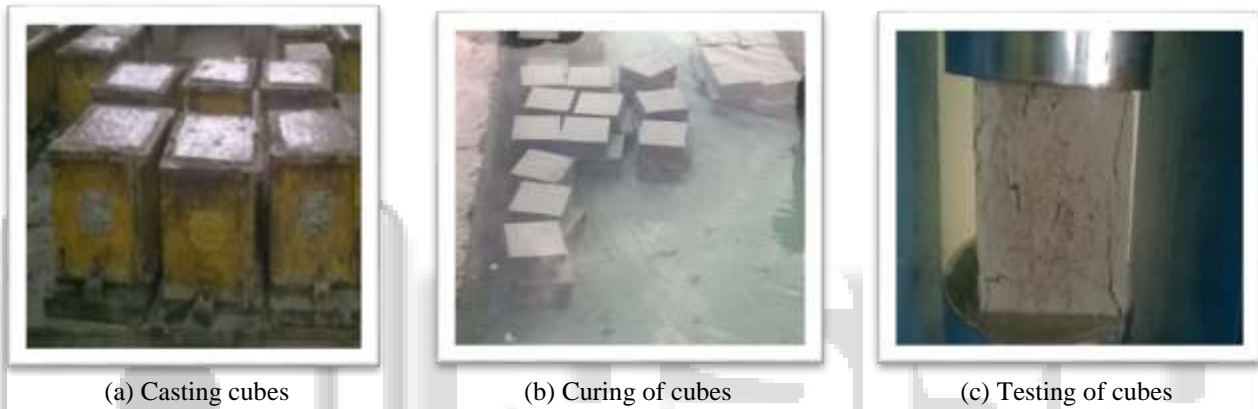
Fig. 3.1: casting and check the compressive strength of cubes
