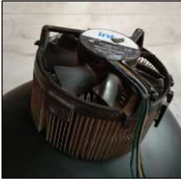
Fig. 9: Side view of helmet with heat sink and electrical fan
