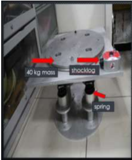
Fig. 4: Single degree of freedom system SDOF system has 4 springs, Each spring has stiffness of 15N/mm with mass of 40 kg
