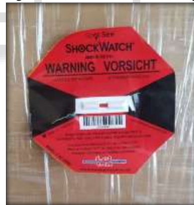
Fig. 2: It turns into red at 50g
