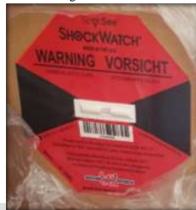
Fig. 1: Shock detector sticker of 50g
