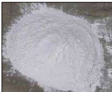
Specific gravity of phosphogypsum is 3.2 Fig. 1: Phosphogypsum
