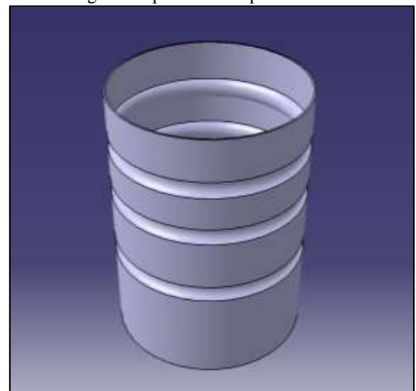
Fig. 3: Circular Shape Crash Box
