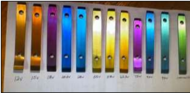
Fig. 1: Titanium Spectrum at different voltage ranges
