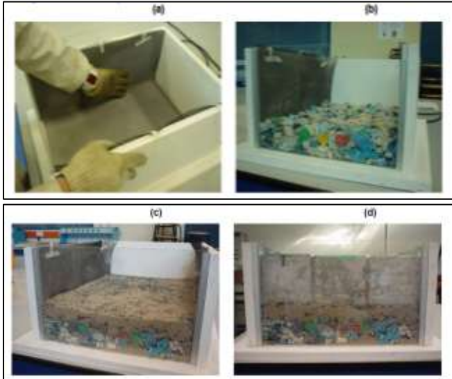
Fig. 3: Construction of the prototype of a permeable interlocking pavement system
