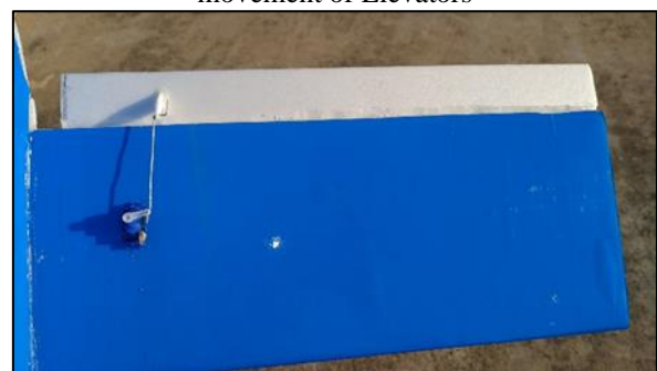
Fig. 10: Positioning of Servo Motor Controlling the movement of right Aileron
