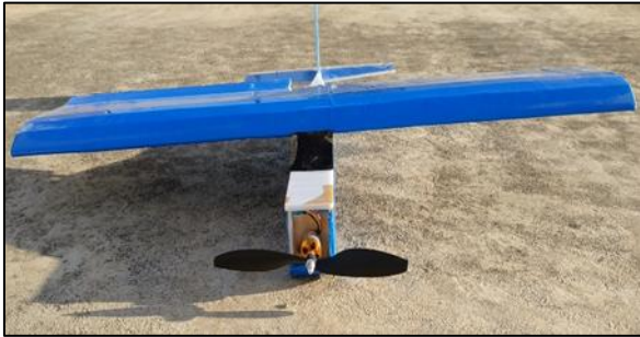
Fig. 12: Attachment of brushless DC Motor & fan blade
