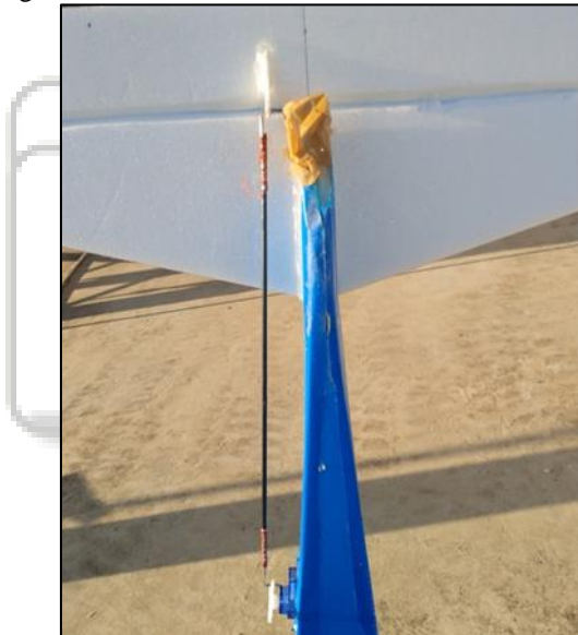
Fig. 13: Addition of extra weight for balancing center of gravity
