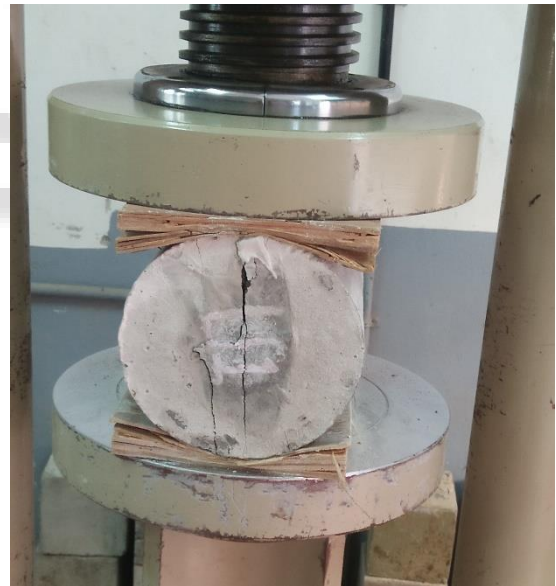
Fig. 3.4: Split Tensile Strength Test
