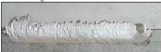
Fig. 6: Defect due to separation of the plates
