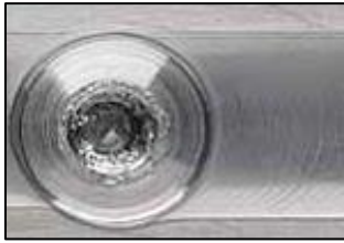
Fig. 5: Defect observed just below the surface of weld in bead on plate weld
