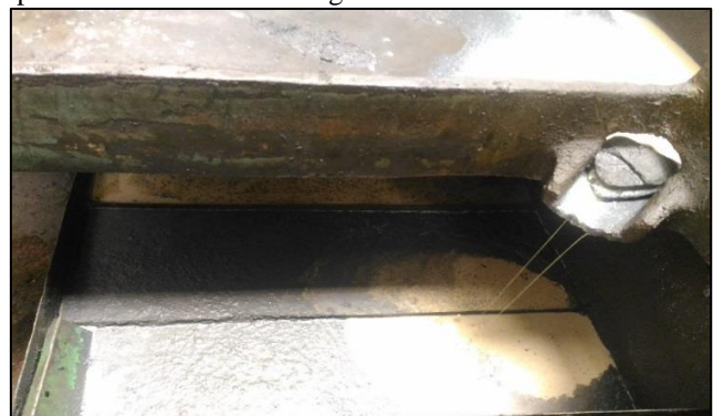
Fig. 2: Mixture of burr and coolant to the recirculating tank
