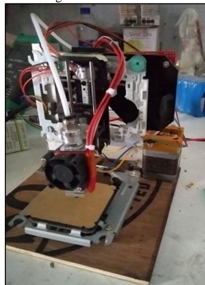
Fig. 2: Assembly of 3D Printer machine using DVD Drive
