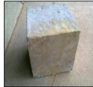
Fig. 2: Concrete cube subjected to sulphate attack
