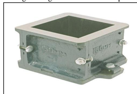
Fig 4.2: Casting Mould (150x150x150)mm
