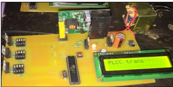
Fig. 4.1: LCD Display of data transmission through PLCC module
