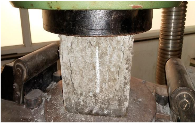
Figure No. 5 Testing of Cube
