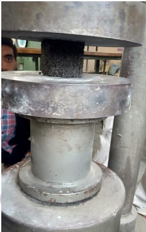
Fig. 1: IMG-Testing of crushed sand mortar
