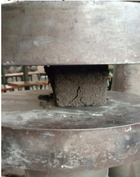
Fig. 2: IMG-Testing of natural sand mortar
