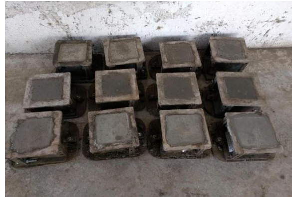
Fig. 4: Finished Concrete cubes
