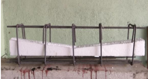
Fig. 2: reinforcement and thermocol used (10% reduction)
