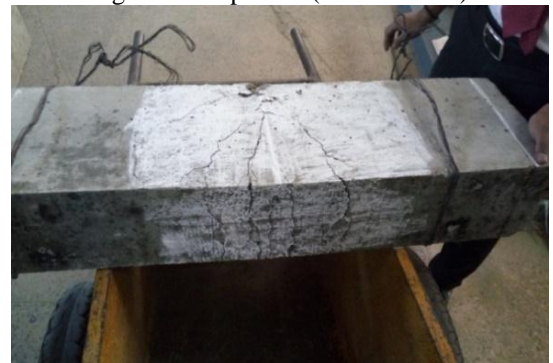
Fig. 6: Crack pattern for control beam
