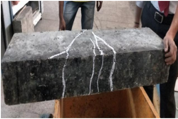
Fig. 7: crack pattern of test specimen (8% reduction)
