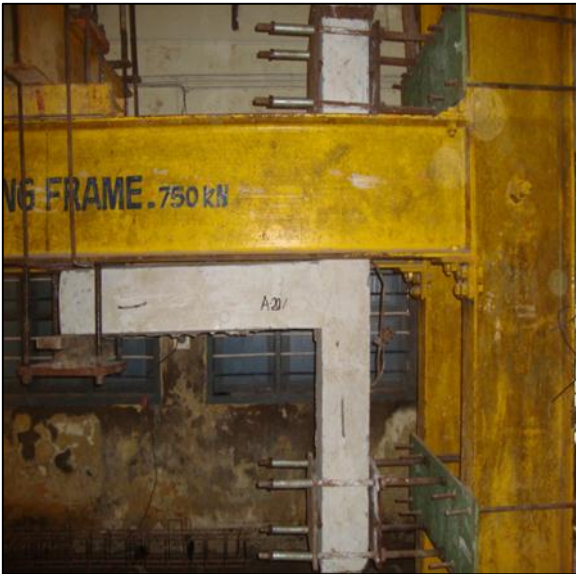
Fig. 5: Typical testing for Non-Ductile joint (IS:456-2000)
