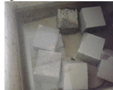
Fig 2. Curing of Cubes
