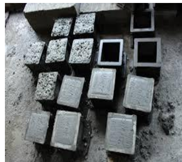
Fig 1. Cube moulds with Concrete
