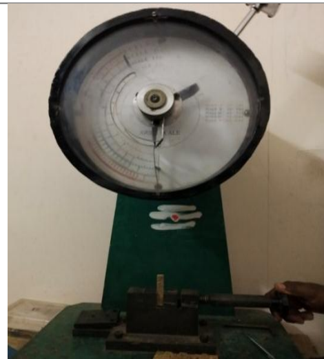
Fig. 5: Impact Test Specimen before Testing
