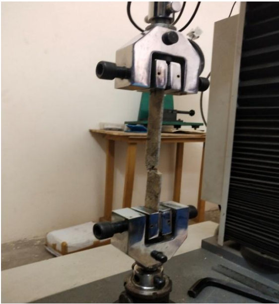
Fig. 2: Tensile Test Specimen after Testing
