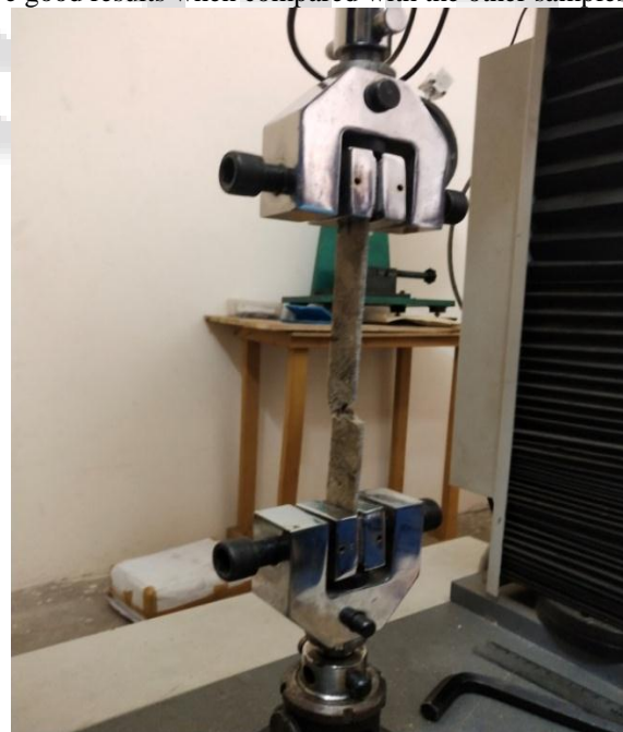
Fig. 1: Tensile Test Specimen before Testing
