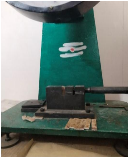
Fig.6: Impact Test Specimen after Testing
