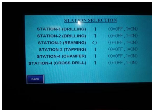
Fig. 4: For selecting a station In the above figure '0' indicates that there is skipping of reaming operation.
