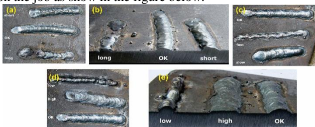
Fig. 1: shows (a)-(b). Arc length Fault (c)-(d). Travel Speed Fault (e). Current Setting Fault[6], [7]
