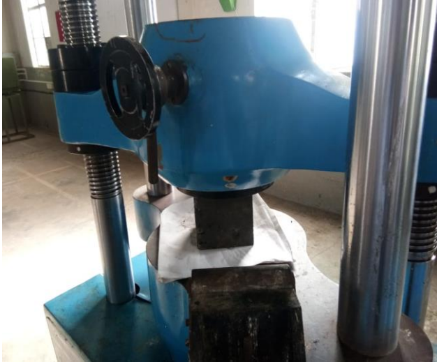
Fig. 1: Compression test on concrete
