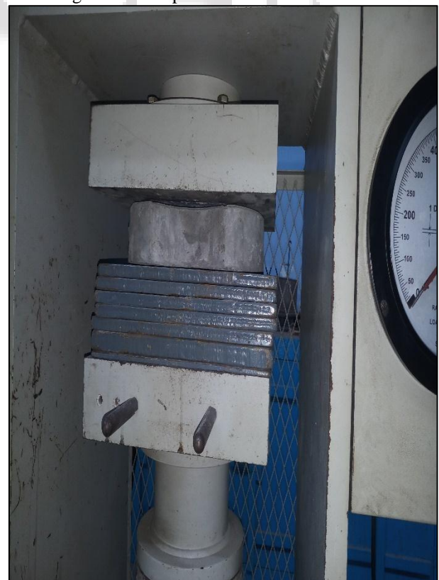
Fig. 5: Compressive strength test
