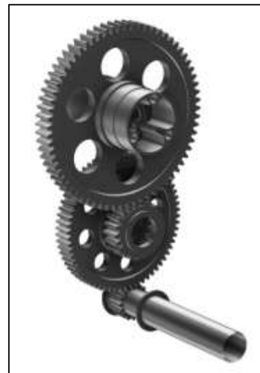
Fig. 2: Cad model of gear train.
