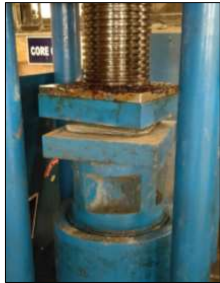
Fig. 4: Compressive strength for plastic sand paver blocks
