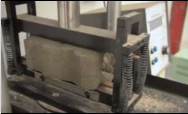
Fig. 5: Flexural strength for plastic sand paver blocks
