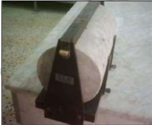
Fig. 3.7.: Testing of Cylindrical Specimen under Split Tensile Strength Test
