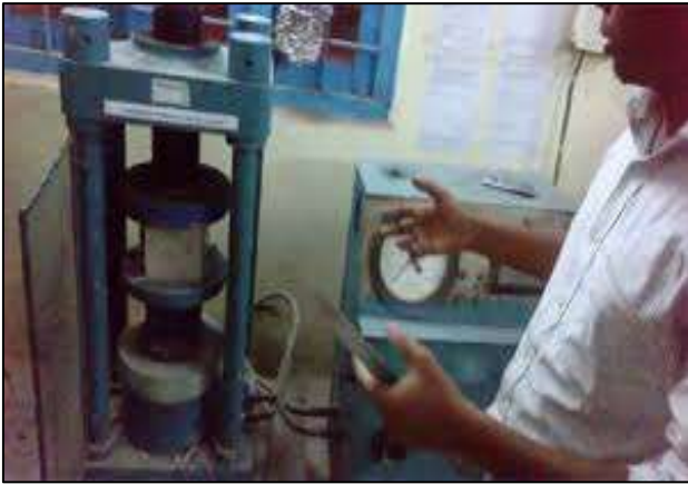
Fig. 3.6.: Testing of cube under compression testing machine
