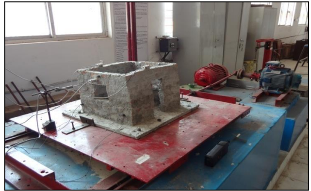
Fig. 3: Building B set up on Shake Table before Test
