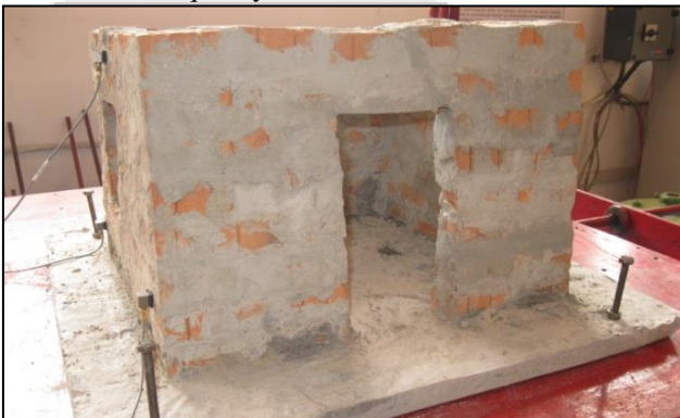
Fig. 2: Building A set up on Shake Table before Test
