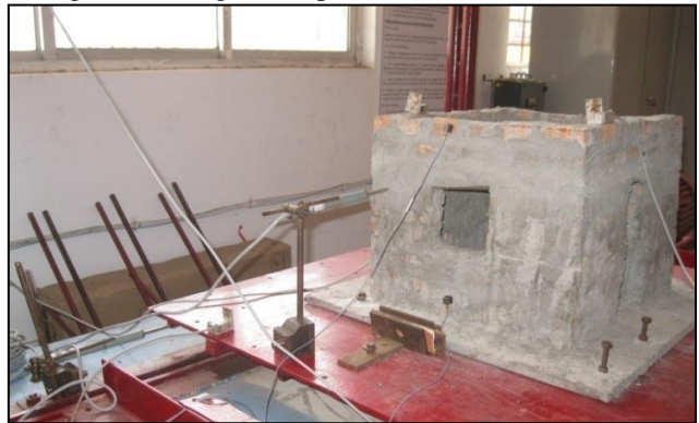
Fig. 4: Building C Set Up on Shake Table before Test
