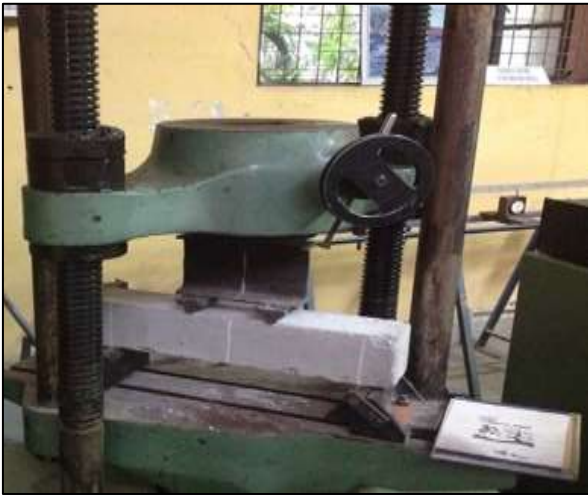
Fig. 7: Experimental Setup for Flexure Test
