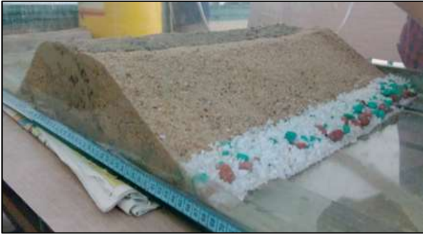
Fig. 2: Model of Zoned type Earth Dam in Transparent Glass Chamber
