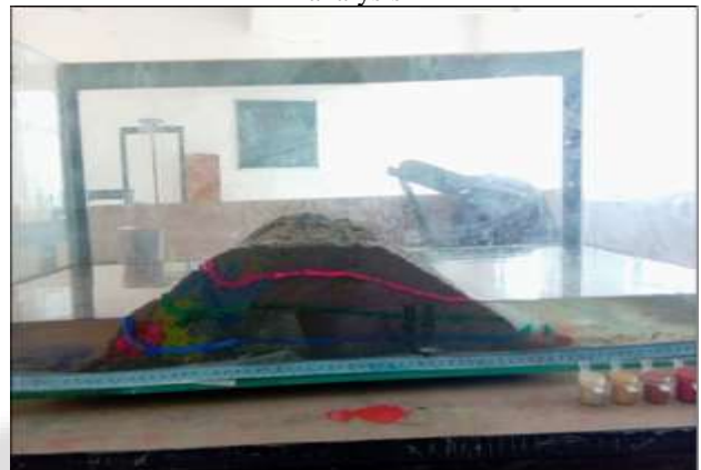
Fig. 6: Phreatic Line or Top Seepage Line when Depth of Water 50 mm, 75 mm, and 100 mm
