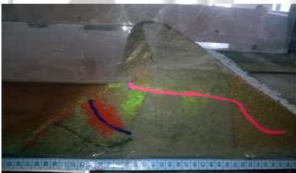
Fig. 6: Phreatic line or top seepage line when depth of water 50 mm, 75 mm, and 100 mm
