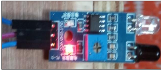
Fig.5. IR sensor is in idle state
