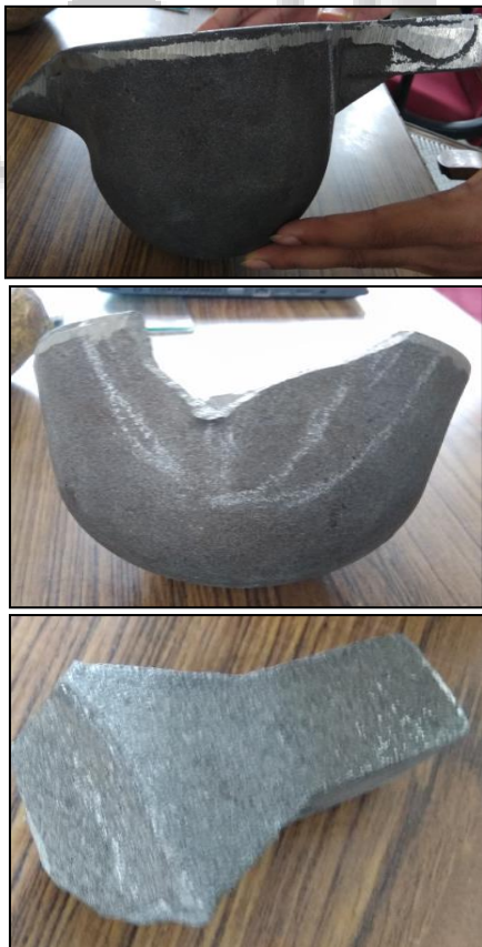
Fig. 1: Actual High Chromium Alloy Cast Iron pouring Ladle ( with and without fracture)
