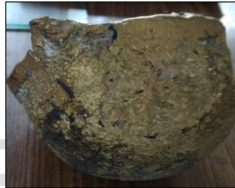
Fig. 9: Cooled molten brass liquid inside pouring cup
