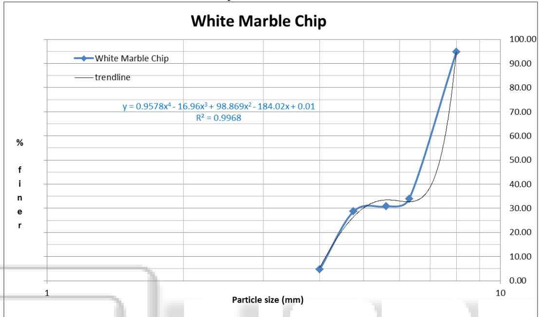
Figure 1: Grain size distribution curve for White Marble Chip
