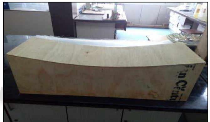
Fig. 1: Wooden mould for making composite leaf spring
