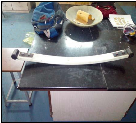
Fig. 3: Mono Composite Leaf Spring
