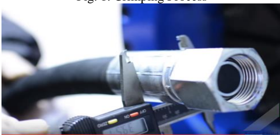
Fig. 2: Crimped Metal Hose & Rubber Tube
