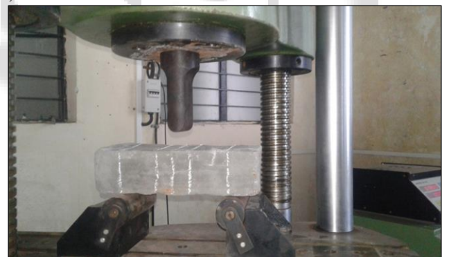
Fig. 6: Flexural Strength Test on EPS Panel The Average Flexural strength of EPS Panel = 5.91 N/mm 2
