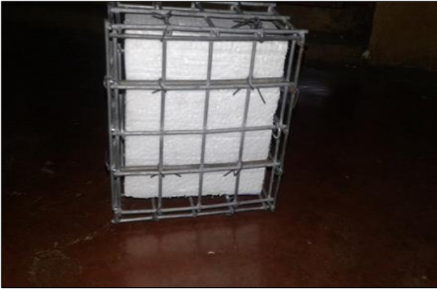
Fig. 1: EPS Panel of size 150mm×150mm×75mm
