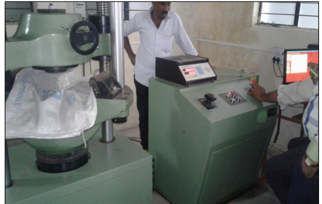
Fig. 5: Compressive Strength Tests on EPS Panels The Average compressive strength of EPS Panel = 3 N/mm 2
