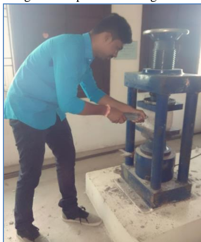
Fig. 3: Rebound Hammer Test
