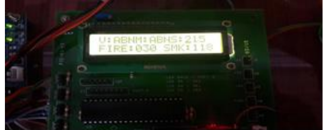
Fig. 4: Abnormal value on LCD
