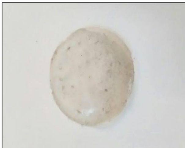
Fig. 6: Potato starch based plastic
