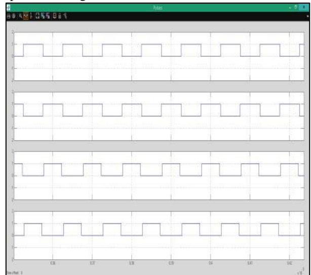
Fig. 8(a): Gate pulses to the switches
