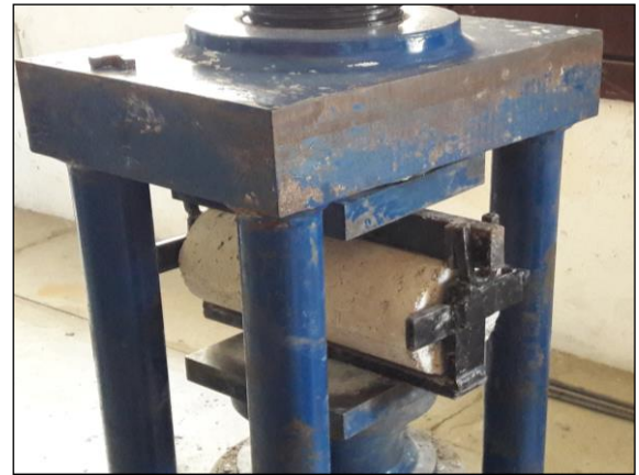
Fig. 2: Set up of a Split tensile strength test
