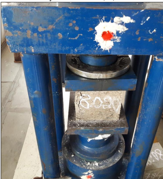
Fig. 1: Set up of a compressive strength test
