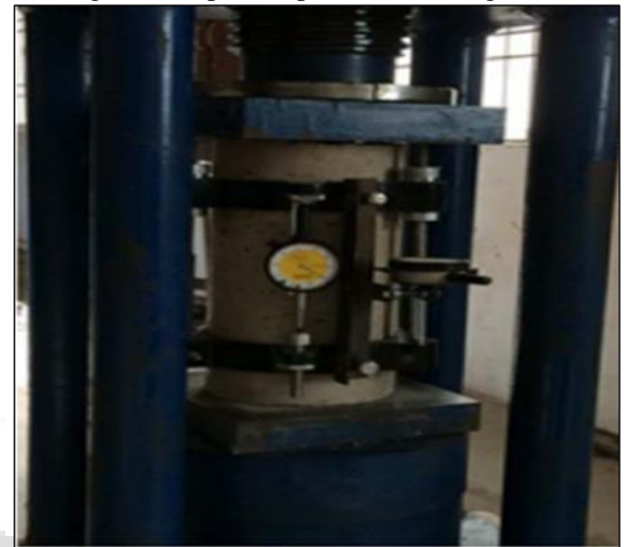
Fig. 3: Set up of a Modulus of Elasticity test
