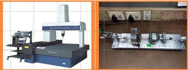
CMM- Which is place measure of Flatness, Roughness, Roundness, cylindricity. Controlling Edge Measuring Instrument: Hook vernier.
