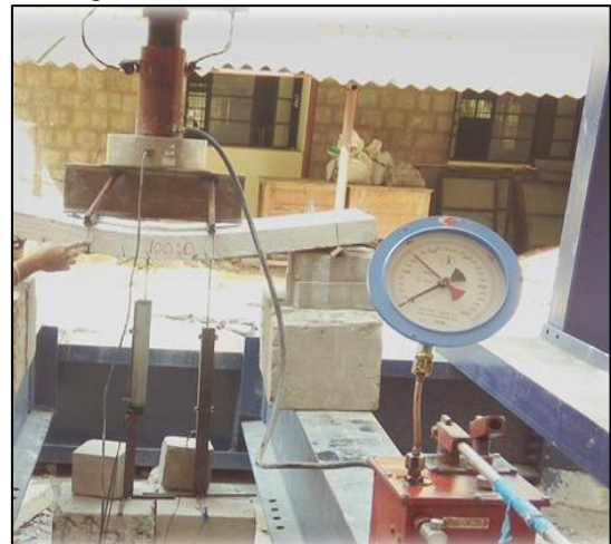
Fig. 1: Set up of a GPC Slab under Two-Point
