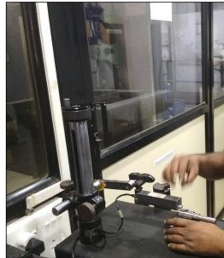
Fig. 5: Surface roughness Tester
