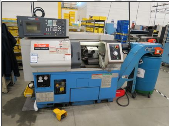
Fig. 3: MAZATROL 640T CNC Lathe
