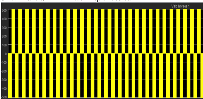
Fig. 22: Inverter output voltage (SVPWM)
